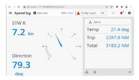
SKIPPER Electronics will in the next few years move all of its products into the Open Bridge platform. This is a browser-based platform where the user interface follows the <a href="https://www.openbridge.no">www.openbridge.no</a> standard interface. This technology uses HTML technology with web
